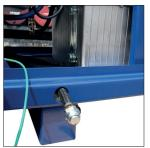
It is recommended to drain the oil while it is at operating temperature. Keep in mind that there is a risk of burn injuries from hot surfaces and possibly from oil at operating temperature. The used oil can be drained into an appropriate container by means of the hose connected to the tank. To do so, remove the plug at the device frame.
